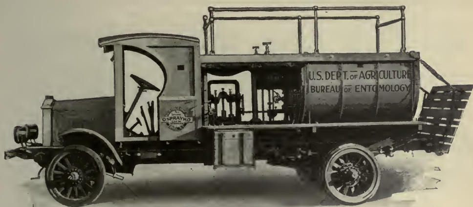
A HIGH-PRESSURE SPRAYER FOR PROTECTING TREES FROM THE RAVAGES OF MOTHS AND OTHER INSECTS
